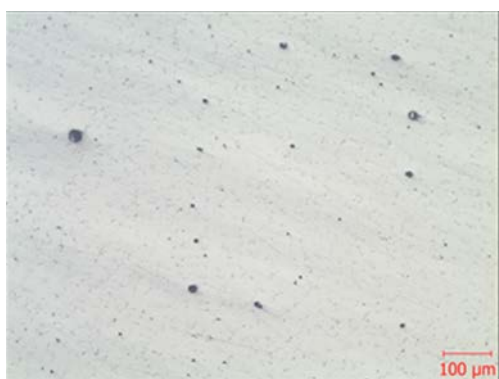
Figure 3. Microstructure of the deposited metal prior to etching
