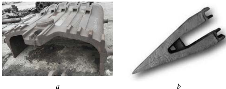
Figure 2. Excavator parts made of 110G13L steel: a – front wall of the excavator bucket; b – excavator bucket tooth
