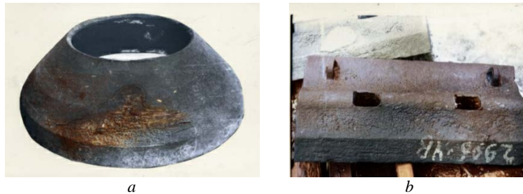
Figure 1. Details of crushing and grinding equipment made of 110G13L steel: a – cone crusher armor; b – ball mill lining
