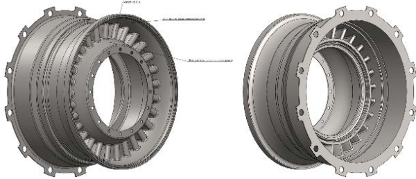
Figure 1. Typical view of a one-part solid-metal NGV of GTE (3D Model)
