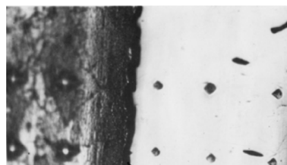
Figure 4. Microstructure of electroplated chromium coating on VD17 alloy
