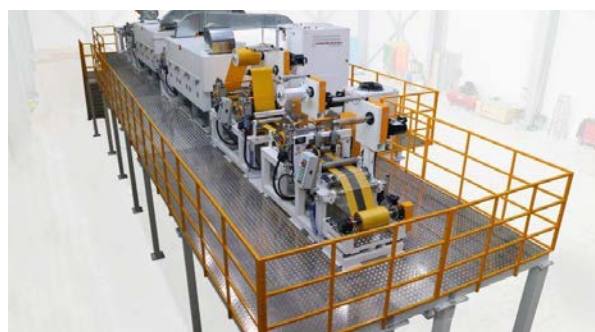
Figure 1. Modular impregnation line for the production of fabric or tow prepregs
