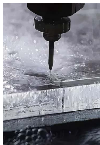
Figure 3. Photo of hydroabrasive cutting
