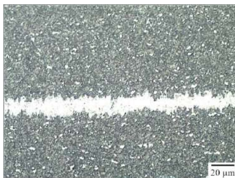
Figure 7. Microstructure of the diffusion bonded joint of nickel-plated 14Cr17Ni2 alloy at T_w = 900\text{ }^{\circ}\text{C} ; P_w = 5\text{ MPa} ; t_w = 35\text{ min}
