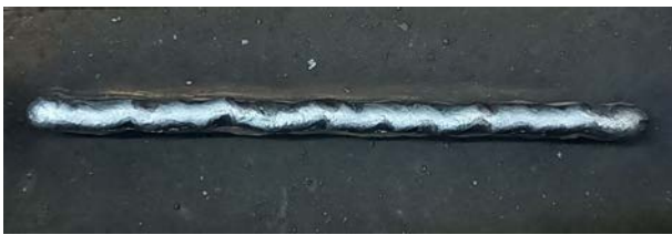
Figure 2. Top view of the 100 % CO 2 deposited wall with severe spatial meandering
