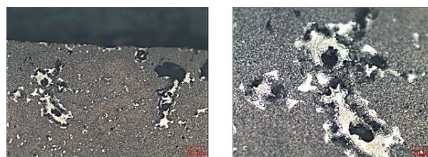
Figure 5. Microstructure of the deposited metal after heat treatment (homogenisation at T=1270\pm 10^\circ\text{C} )
