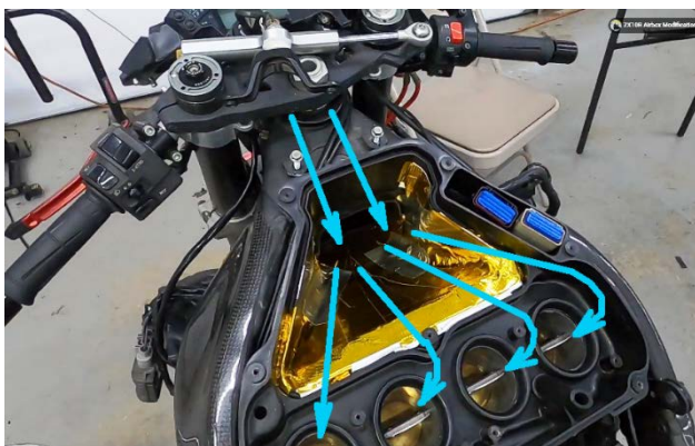
Figure 2. Schematic of the intake system and airflow path in the Kawasaki Ninja ZX-10R motorcycle (air filter not shown) [14]
