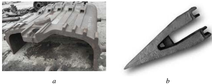
Figure 2. Excavator parts made of 110G13L steel: a – front wall of the excavator bucket; b – excavator bucket tooth
