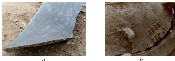
Figure 3. Parts of a cone crusher made of 110G13L steel that have failed: a – worn out armor of the cone crusher; b – crack in the armor of the cone crusher
