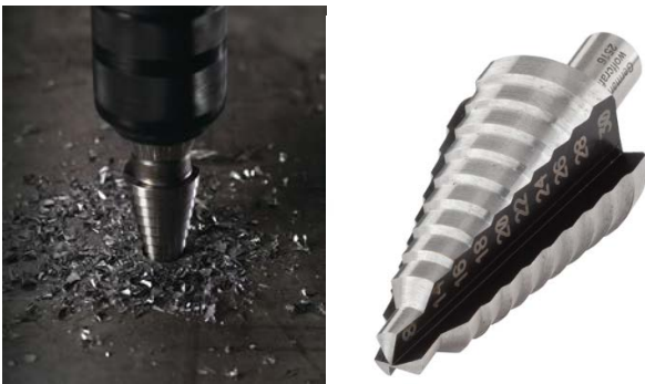
Figure 1. Step drill 8-30 mm
