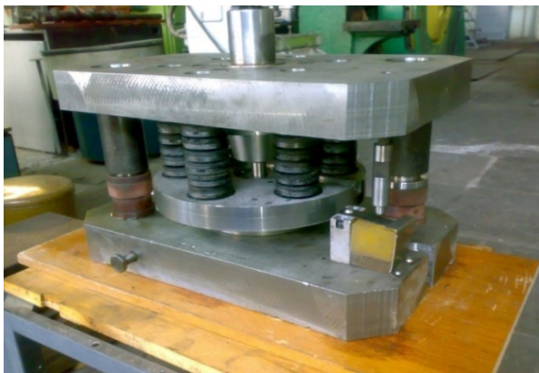
Figure 10. Photo of an experimental stamp for punching a hole
