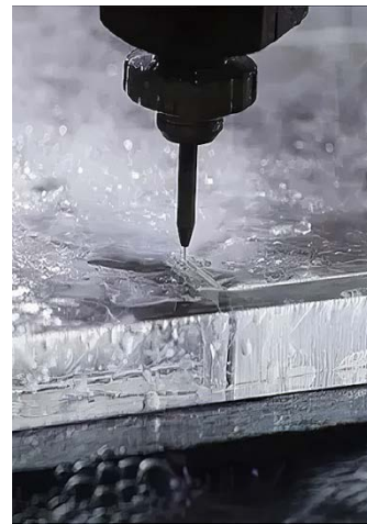
Figure 3. Photo of hydroabrasive cutting
