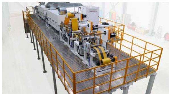
Figure 1. Modular impregnation line for the production of fabric or tow preregs
