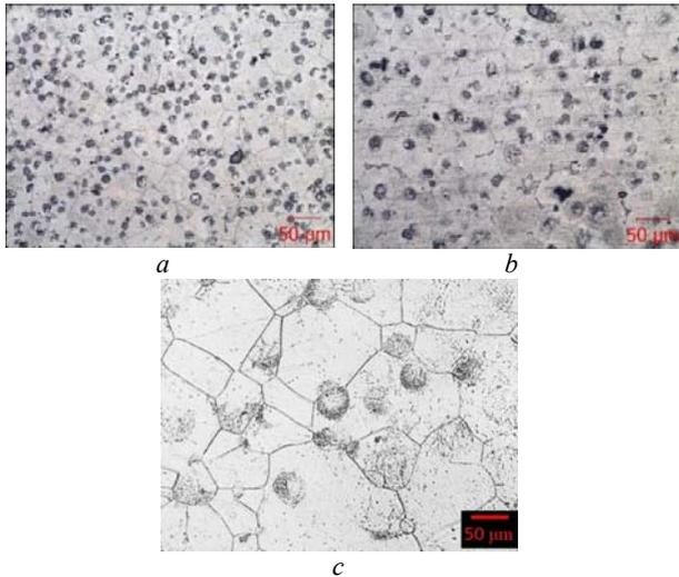
**Figure 8.** Microstructures of the studied alloys after aging,  $\times 200$ : developed alloy processed using the new mode (a), developed alloy processed by the standard mode (b), standard Mg-2.5Nd-0.4Zn-0.5Zr (wt%) alloy, processed according to the standard mode (c)
