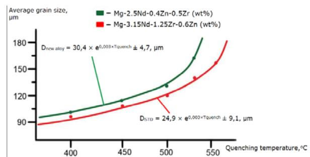
**Figure 7.** Dynamics of changes in the average grain size of experimental alloys at different heating temperatures for quenching
